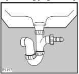
Push the drain hose onto the spigot and secure with a clip if required, ensure a loop is formed in the drain hose (see diagram) to prevent waste from the sink entering the washing machine.
